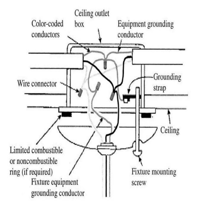
(3) Where lighting fixtures are mounted on combustible surfaces such as hardboard, a limited combustible or noncombustible ring, as shown in figures 7A and 7B of this rule, shall be installed to completely cover
