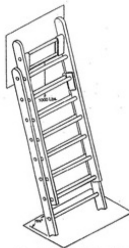
Figure 3 Extension ladder positioned for hardware test.
