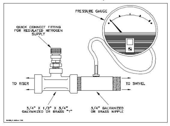
Vapor Coupler Integrity Assembly. Assemble OPW 633-A, 633-B, AND 634-A adapters, or equivalent, as shown in Figure 2. If the test is to be conducted at the storage tank Stage I vapor coupler, this assembly shall be used prior to conducting the static leak test in order to verify the pressure integrity of the vapor poppet. The internal volume of this assembly shall not exceed 0.1 cubic feet.
