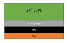
(2) Cap over disposed waste generally having a permeability less than 1 x 10<sup>-5</sup> cm/sec:
